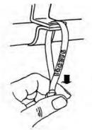
3. Gently pull on seal to insure it is securely locked.
