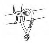
2. Firmly insert end into locking device until lock is engaged.
