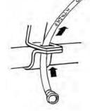
Place flat end of seal through opening of locking mechanism. Bend strip to locking device at opposite end of seal.
